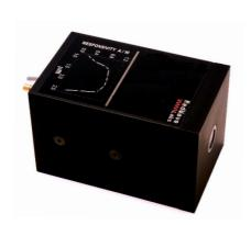
The D123 is an amplified extended InGaAs photoreceiver for the detection of light in the spectral range 900–2500nm. An integrated temperature controller maintains the D123 temperature at -25°C for low noise operation. Three mounting holes allowing pure rotation of the diode, eliminating unwanted translation during mounting.
